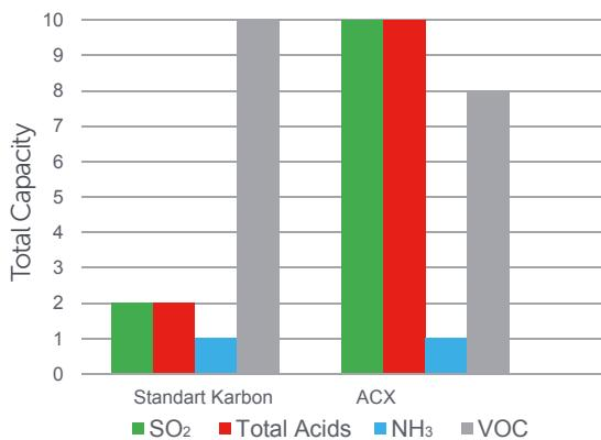
ACX Carbon media test - tracer gas SO<sub>2</sub>
